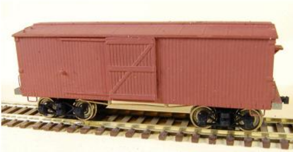
The car with Panamint Models HOT71s "Cleveland" 4'-10" wheelbase archbars from Shapeways in "Black Strong & Flexible".
